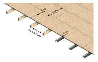
When installing the floor board, the temperature and relative humidity in the building must be close to the future use conditions. The frame structure must also be sufficiently dry. The chipboard must be stored in a clean and dry place (RH<60%) and conditioned close to the future use conditions for 5 to 7 days before use.
