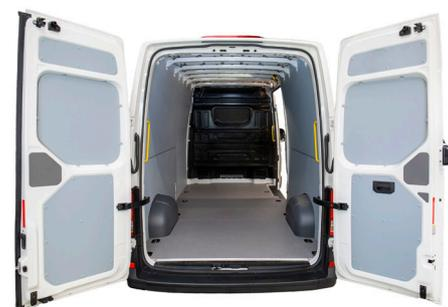
The panels protect the cargo space from scratches and dents during everyday work and allow it to be kept tidy and hygienic
